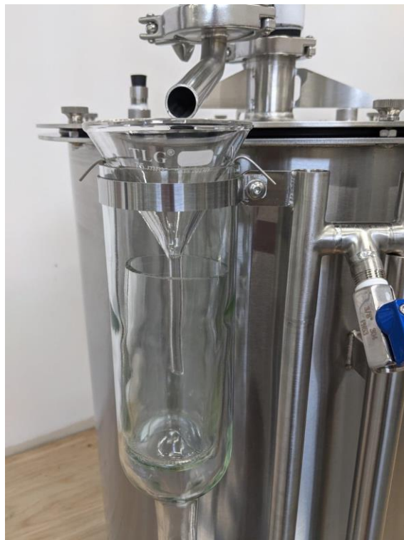
4: Florentine flask for heavy oils (with glass funnel and glass flask inside)
