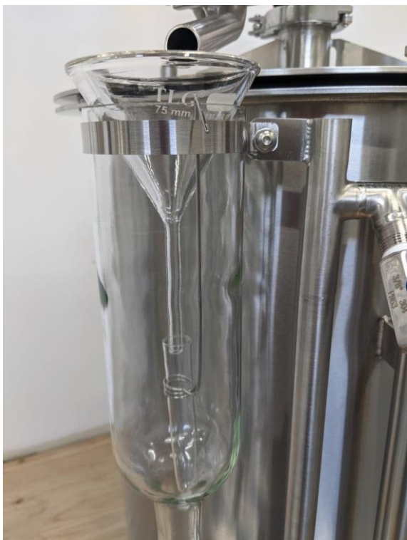
3: Florentine flask for light oils (with glass funnel and coiled tube)
