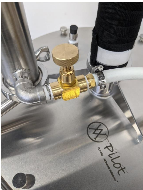
1: Hose fastening on the inlet barbed fitting
