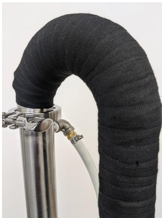
2: Hose fastening on the outlet barbed fitting
