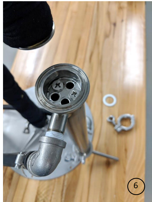
Condenser restriction with conical-head screws (no more than 2 tubes!)
