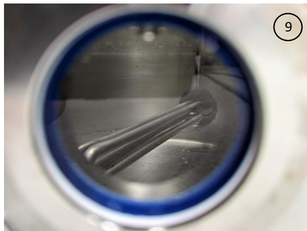
Electric heating element installed in the Explorer with the regulator and the sight glass at the bottom of the tank
