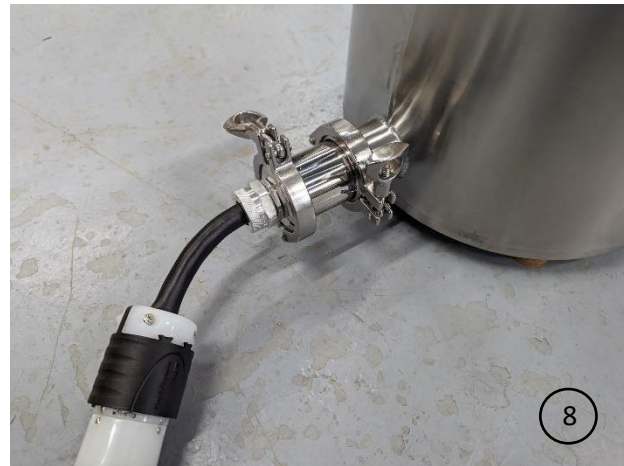
Condenser restriction with conical-head screws (no more than 2 tubes!)
