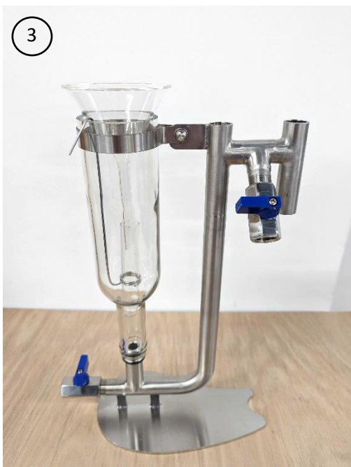
Florentine flask for light oils With glass funnel and glass tube
