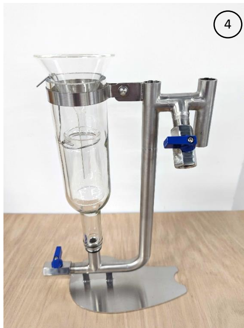
Florentine flask for heavy oils With glass funnel and glass flask
