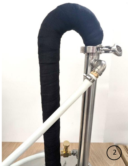
Hose fastening on the outlet barbed fitting
