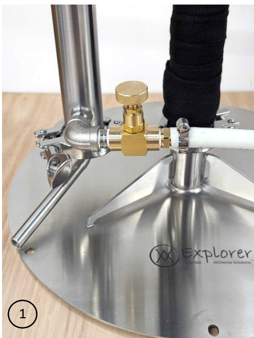
Hose fastening on the inlet barbed fitting
